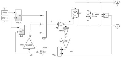
Fig.16 The electrical Matlab model of a PV module.
