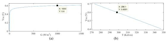
Fig.11 The influence of solar irradiation and temperature on the value of the open circuit voltage; (a) the influence of solar irradiation, (b) the influence of temperature.
