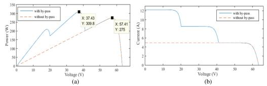
Fig.18 The characteristics of PV array under partial shading conditions(a) V-P characteristic, (b) V-I characteristic.
