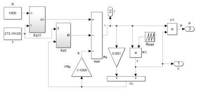
Fig.5 The Matlab model of the PV cell.
