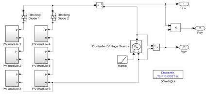
Fig.17 PV array model.
