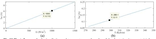
Fig.10 The influence of solar irradiation and temperature on the value of the short-circuit current; (a) the influence of solar irradiation, (b) the influence of temperature.
